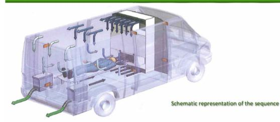
The MIESEN Infection ambulance is based on a box-type van and equipped with a special ventilation and filtering technique, which allows to transport highly contagious patients without any danger for the surrounding population.
