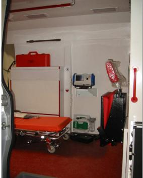
The concept of this ambulance is primarily focussed on the transport of highly infectious (contagious) patients without risk to the environment. This is realized by a constant negative pressure in the patients compartment and filtration of exhaust air through high efficiency filters.
