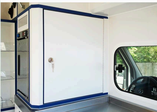
Ampullenschrank an der Trennwand Cabinet for ampoules situated at the partition wall
